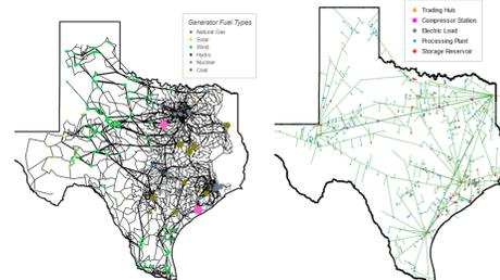
Fig. 3: Combined transmission and gas network for the Texas-7k case.
